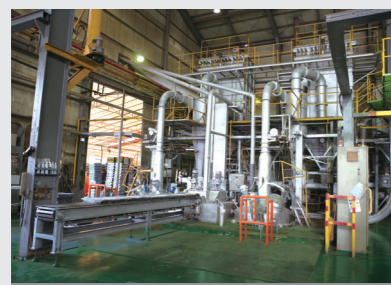
Lead Powder Process Ingot Melting → Primary Oxidation
