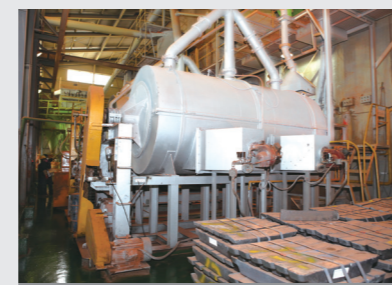
Red Lead Process Primary Oxidation (Lead Powder) → Secondary Oxidation
